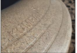
The sand colored variant is made of rotomolded stone mixed PE made from 33% post consumer materials with a non skid surface texture. Minor differences in the stone mix visuality of the material are to be expected.
