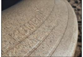
The sand colored variant is made of rotomolded stone mixed PE material with non skid surface texture. Minor differences in the stone mix visuality of the material are to be expected.
