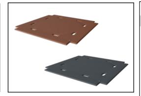
Floors and panel activities are available in two types of material: Waterproof plywood decks thickness 21.5mm from pine and alder wood with anti-slip film on both sides. High Pressure Laminate HPL thickness 17.8mm with slip resistant surface texture according to EN 438-6.
