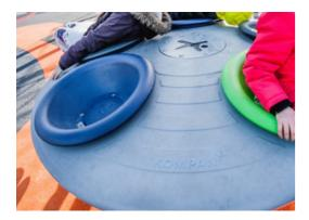
The Multispinner grey base is made of recyclable PE. The base is moulded in one piece with integrated metal thread bushings and water drain holes to ensure high durability in all climates around the world. Each bowl is mounted separately into the base.
