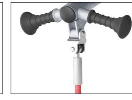
The two angled top handles are made of a moulded PP insert with an outer soft layer of TPV rubber. The handle is attached to the pipe with a galvanised steel inlay to ensure strength and durability.
