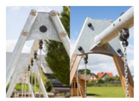
The A-Frame is designed with hot dip galvanised ø100mm crossbar with large steel end plates for strong fixation of the two post options: Hot dip galvanised ø70mm steel. Impregnated pine wood with hot dip galvanised steel footings.
