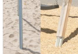
The post of the A-Frame swings are available for surface anchoring with expansion bolts or inground in 60cm or 90cm depth. The hot dip galvanised steel legs are anchored directly in the ground. Pine wood posts are elevated from ground by a unique profiled hot dip galvanised steel footing.
