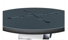
The ø414mm top plate is made from 15mm Ekogrip®, a 15mm PE plate with a 3mm toplayer of thermoplastic rubber with non-skid effect. The height is 217mm and the range of motion is +/- 90?, with a EPDM rubber stop at each end.
