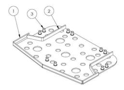
A 5 mm hot-dip galvanised carbon steel plate must is moulded inside the SBR to offer optimal stability and optimize the mounting of the step to the frame.
