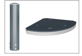
ELEMENTS decks are made of 17,8mm thick HPL supported by a unique designed aluminum frame with multiple attachment options by usage of aluminum connectors. The main posts are made of high quality pre-galvanized steel with powder coated top finish. Post tops are closed with caps of UV stabilised nylon (PA6).
