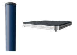
ELEMENTS decks are made of 17.8mm thick HPL supported by a unique designed aluminum frame with multiple attachment options by usage of aluminum connectors. The main posts are made of high quality pre-galvanised steel with powder coated top finish. Post tops are closed with plastic caps of UV stabilised nylon PA6.
