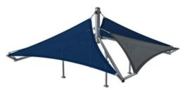
Sails of commercial 95 high density PE knitted specially for sun-shade structures. The sails are treated with UV stabilizers to ensure a long lifetime. The sails are supported by a hot dip galvanized steel frame and tightened by stainless steel devices.
