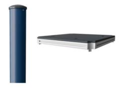
ELEMENTS decks are made of 17.8mm thick HPL supported by a unique designed aluminum frame with multiple attachment options by usage of aluminum connectors. The main posts are made of high quality pre-galvanised steel with powder coated top finish. Post tops are closed with plastic caps of UV stabilised nylon PA6.
