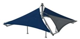
Sails of commercial 95 high density PE knitted specially for sun-shade structures. The sails are treated with UV stabilizers to ensure a long lifetime. The sails are supported by a hot dip galvanised steel frame and tightened by stainless steel devices.
