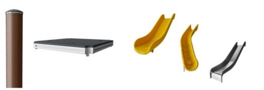
ELEMENTS decks are made of 17.8mm thick HPL supported by a unique designed aluminium frame with multiple attachment options by usage of aluminium connectors. The main posts are made of high quality pre-galvanised steel with powder coated top finish. Post tops are closed with caps of UV stabilised nylon (PA6).
