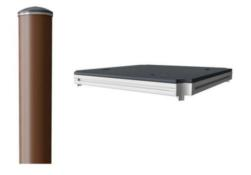
ELEMENTS decks are made of 17.8mm thick HPL supported by a unique designed aluminium frame with multiple attachment options by usage of aluminium connectors. The main posts are made of high quality pre-galvanised steel with powder coated top finish. Post tops are closed with caps of UV stabilised nylon (PA6).
