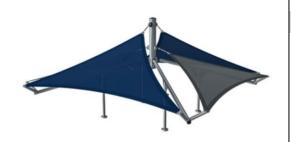
Sails of commercial 95 high density PE knitted specially for sun-shade structures. The sails are treated with UV stabilizers to ensure a long lifetime. The sails are supported by a hot dip galvanised steel frame and tightened by stainless steel devices.
