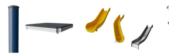
ELEMENTS decks are made of 17.8mm thick HPL supported by a unique designed aluminium frame with multiple attachment options by usage of aluminium connectors. The main posts are made of high quality pre-galvanised steel with powder coated top finish. Post tops are closed with caps of UV stabilised nylon (PA6).
