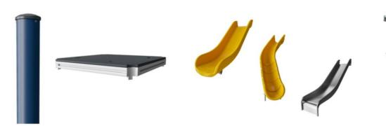
ELEMENTS decks are made of 17.8mm thick HPL supported by a unique designed aluminium frame with multiple attachment options by usage of aluminium connectors. The main posts are made of high quality pre-galvanised steel with powder coated top finish. Post tops are closed with caps of UV stabilised nylon (PA6).
