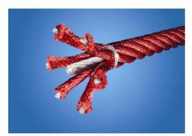
Corocord ropes with 19 mm diameter or more are special "Hercules" – type with galvanised six–stranded steel wires. Each strand is tightly wrapped with PES yarn, which is melted onto each individual strand. The ropes are highly wear-and vandalism-resistant and can be replaced at site if needed.
