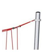
Corocord ropes with 19 mm diameter or more are special "Hercules" – type with galvanised six–stranded steel wires. Each strand is tightly wrapped with PES yarn, which is melted onto each individual strand. The ropes are highly wear-and vandalism-resistant and can be replaced at site if needed. The steel posts are hot dip galvanised inside and outside with lead free zinc. The galvanisation has excellent corrosion resistance in outside environments and requires low maintenance.
