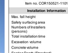
Installation Information Max. fall height 265 cm Safety surfacing area 48.6 m<sup>2</sup> Numbers of Installers 2 Total installation time Excavation volume 4.31 m<sup>3</sup> Concrete volume 2.74 m<sup>3</sup> Footing Depth (Standard) 110 cm Shipment Weight 312 kg Anchoring options In-ground
