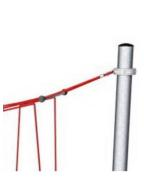
Corocord ropes with 19 mm diameter or more are special "Hercules" – type with galvanised six–stranded steel wires. Each strand is tightly wrapped with PES yarn, which is melted onto each individual strand. The ropes are highly wear-and vandalism-resistant and can be replaced at site if needed. The steel posts are hot dip galvanised inside and outside with lead free zinc. The galvanisation has excellent corrosion resistance in outside environments and requires low maintenance.
