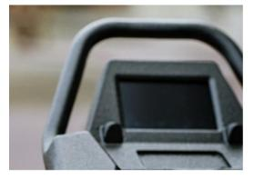
The handle bars is designed with multiple hand positions to accommodate different postures and riding styles. It is a casted Aluminum part with Polyurea coating for good grip and insulation.
