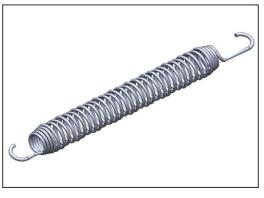
All 72 springs are made of stainless steel to ensure durability and excellent corrosion resistance. The steel wire is 3,2 mm thick and the last five windings are cone shaped to ensure long lifetime of the jumper.
