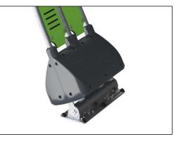
The rocking movement back and forth is controlled by a heavy duty scaled double rubber torsion spring element. The rubber element ensures a safe movement and reduces speed towards the tower platforms. The base cover of molded PE material with high impact resistance.
