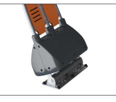
The rocking movement back and forth is controlled by a heavy duty scaled double rubber torsion spring element. The rubber element ensures a safe movement and reduces speed towards the tower platforms. The base cover of molded PE material with high impact resistance.
