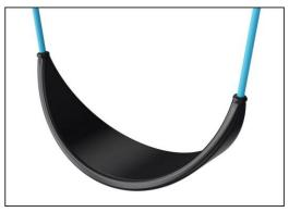
The belt seat is made of UV stabilized PUR. It retains its properties in the temperature range of -30°C to 60°C. The ropes are made of UV-stabilized PP rope with inner steel cable reinforcement and outside layer of transparent PUR.
