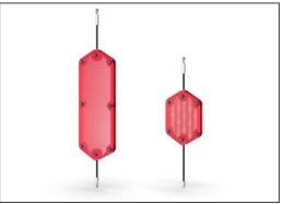
Turnable optic panels of two 7mm thick polycarbonate plates with a distance of 25mm. The inside graphic print consist of an inner image layer and outer transparent protection layer. Both PC panel and the water-based lacquer are UV stabilized to prevent fading of the print.
