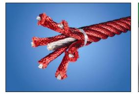
Corocord ropes with 19mm diameter or more are special 'Hercules' - type with galvanised sixstranded steel wires. Each strand is tightly wrapped with PES yarn, which is melted onto each indivudual strand. The ropes are highly wear-and vandalism-resistant and can be replaced at site if needed.
