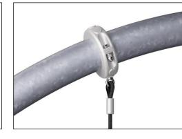
Corocord aluminium clamps are used as connectors between steel posts and rope. Two aluminium castings are bolted together. The height of the clamps is thus variable.
