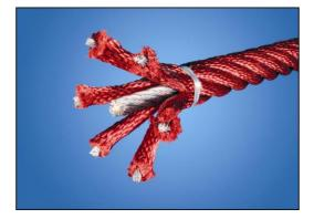
Corocord ropes with 19mm diameter or more are special 'Hercules' - type with galvanized sixstranded steel wires. Each strand is tightly wrapped with PES yarn. The ropes are connected by stainless steel S-Clamps which are pressed around the rope which results in a durable and vandalism solution.
