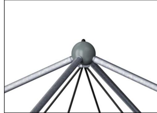
The unique designed connector balls with a diameter of 230mm are made of high quality aluminum with a powder coated top finish. The inside tensioning parts are made of hot dip galvanized steel.
