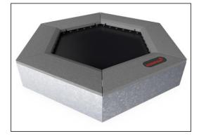
All steel components are manufactured from carbon steel S235 in a thickness of 3 mm. Side panels, support walls for top frame, plates bended with SBR and plates flat for in-situ surfacing are hot dip galvanized.
