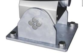
The double ROSTA element is made of casted iron and hot dip galvanised before painted. This ensures that the ROSTA element is a maintenance free, elastic joint which can be move in range of motion is 250 in any direction. Both wobbles have a different stiffness, difference is 45%.
