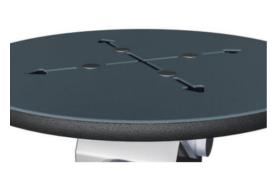
The bearings used in the Twist are slide bearings made of polyoxymethylene, a material that has all the properties needed for a strong bearing: extremely low wear, high mechanical strength, Low moisture absorption and High abrasion resistance. The ø414mm top plate is made from 15mm Ekogrip®, a 15mm PE plate with a 3mm toplayer of thermoplastic rubber with non-skid effect. The height is 217mm and the range of motion is +/- 90?, with a EPDM rubber stop at each end.
