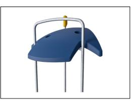
The ELEMENTS roofs are made of recyclable PE with a minimum wall thickness of 5 mm to ensure high durability in all climates around the world. The steel pipes are hot dip galvanised inside and outside for maximum durability.
