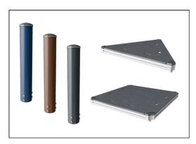
The main posts are made of high quality pregalvanized steel with powder coated top finish. Post tops are closed with caps of UV stabilized nylon (PA6). The grey colored molded decks are made of 75% post-consumer ocean waste PP material with a non-skid pattern and texture surface. All decks are supported by unique designed low-carbon aluminum profiles with multiple attachment options.
