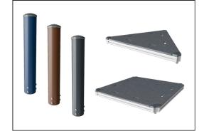
The main posts are made of high quality pregalvanized steel with powder coated top finish. Post tops are closed with caps of UV stabilized nylon (PA6). The grey colored molded decks are made of 75% post-consumer ocean waste PP material with a non-skid pattern and texture surface. All decks are supported by unique designed low-carbon aluminum profiles with multiple attachment options.
