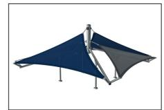
Sails of commercial 95 high density PE knitted specially for sun-shade structures. The sails are treated with UV stabilizers to ensure a long lifetime. The sails are supported by a hot dip galvanised steel frame and tightened by stainless steel devices
