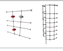
Ropes are made of UV-stabilized PES rope strands with inner steel cable reinforcement. The polyester wrapping is inductively melted onto each strand to obtain excellent wear and tear resistance.
