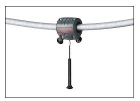
The hang-on puller is designed with at welded steel core and covered with low-density PE housing. The two hot dip galvanised steel handles are angled to provide best possible ergonomic while gliding. The wheels of the puller are made of low noise TPU and installed with sealed ball bearings.
