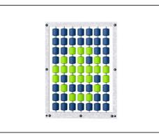
The two colored turnable rollers are made of high quality UV stabilized and reinforced nylon (PA). The rollers are assembled on vertical steel pipes in a welded frame. All steel parts are hot dip galvanized.
