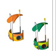
Max. fall height 100 cm Safety surfacing area 36.6 m<sup>2</sup> Number of installers Total installation time 19.3 **Excavation volume** 0.69 m<sup>3</sup> Concrete volume 0.28 m<sup>3</sup> Footing depth (standard) 60 cm 568 kg Shipment weight Anchoring options Surface In-ground **Warranty Information** FcoCore HDPF Lifetime Post 10 years PP Decks 10 years 10 years Ropes & nets
