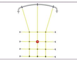
ELEMENTS ropes has six-stranded steel wires and a steel wire core. Each strand is tightly wrapped with PES yarn, which is made from +95% post consumer materials. The yarn is then melted onto each individual strand making the ropes highly wear- and vandalism-resistant.
