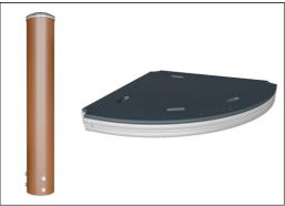
ELEMENTS decks are made of 17.8mm thick HPL supported by a unique designed aluminum frame with multiple attachment options by usage of aluminum connectors. The main posts are made of high quality pre-galvanised steel with powder coated top finish. Post tops are closed with caps of UV stabilised nylon (PA6).
