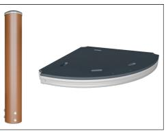
ELEMENTS decks are made of 17.8mm thick HPL supported by a unique designed aluminum frame with multiple attachment options by usage of aluminum connectors. The main posts are made of high quality pre-galvanised steel with powder coated top finish. Post tops are closed with caps of UV stabilised nylon (PA6).
