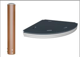
ELEMENTS decks are made of 17.8mm thick HPL supported by a unique designed aluminum frame with multiple attachment options by usage of aluminum connectors. The main posts are made of high quality pre-galvanised steel with powder coated top finish. Post tops are closed with caps of UV stabilised nylon (PA6).
