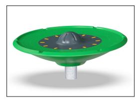
The outer ring of the Spinner Disc base is made of recyclable LDPE. The ring is molded in one piece with integrated metal thread bushings and water drain holes to ensure high durability in all climates around the world.
