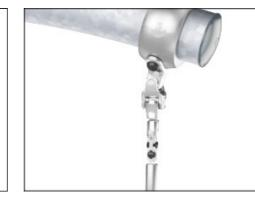
The swing hangers are made of stainless steel brackets and can move over two axis. The flange bearings are silicone enriched to make the suspension maintenance free. The connection to the rope is made with stainless steel chain.
