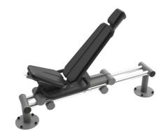
The seat and head support are made of Polyurethane Rubber and have a steel insert plate that connects it to the steel frame. The seat is adjustable in 14 different settings to fit users from 140/ 205 cm tall and to vary the type of exercises. The seat is positioned under a 12degree angle and the back supports a 48degree angle. The back support has a groove, accommodating a comfortable position.
