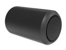
The rotating rollers are  $\emptyset$  110mm and made from PUR (Polyurethane Rubber, compact foam). The rollers have a steel insert that is electro galvanized. They provide support and ensure a comfortable position.
