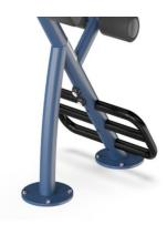
All Steel components are made from carbon steel, with a hot-dip galvanized surface according to ISO1461, and a powder coating corrosion class C3 according to ISO12944-2. Lead content for surfaces is below 90ppm, and below 100ppm for base material.
