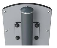
The connectors are made of die-cast aluminum specially alloyed for outdoor environments and with a lead content below 100ppm. The connectors are attached to the posts by stainless steel screws and well protected against corrosion by special designed zinc washers. Extremely strong and no change of corrosion.
