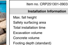
Max. fall height 240 cm Safety surfacing area 62.4 m<sup>2</sup> Total installation time 16.1 Excavation volume 10.58 m<sup>3</sup> Concrete volume 5.88 m<sup>3</sup> Footing depth (standard) 90 cm Shipment weight 599 kg Surface Anchoring options In-ground
